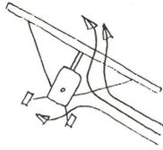
Dihedral works in 2 ways. One is the low wing has more vertically directed lift than the high wing.
