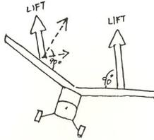
But that's only a small part. The biggest is that air flowing against the side of the nose in the sideslip flows up the fuselage to strike the low wing. The wing "feels" this as an increased angle of attack (the air flow is hitting the airfoil on the chin instead of the nose) and consequently produces more lift than its mate.
