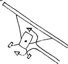
However, look what happens if you put a clear plastic forward fin between the wing and the fuselage. The upward sliding air is forced up against the low wing and you get roll out instead of roll off!!
