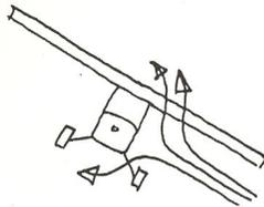
Now you can see why low wings are so spirally unstable. The airflow slides down the fuselage to hit the wing at a downward angle. The wing "feels" this as a lesser angle of attack and produces less lift than its mate and over she goes!
